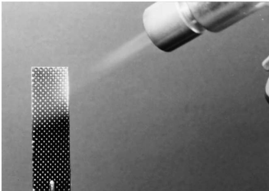
Figure 4 Combustion test of the CFRP using MSP. (non combustible and smokeless).
