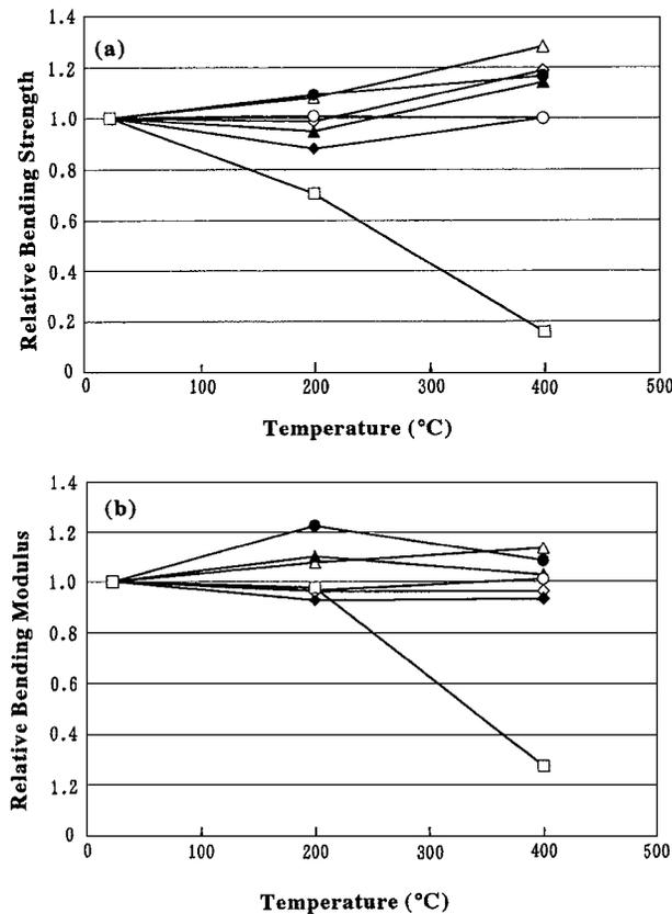
Figure 5 Changes of the bending strength (a) and modulus (b) with the measuring temperature. FRPs were cured at 400°C (opened mark) or 600°C (closed mark). (Δ) CFRP, (○) SiCFRP, (◇) GFRP, (□) FRP (PMR-15).
