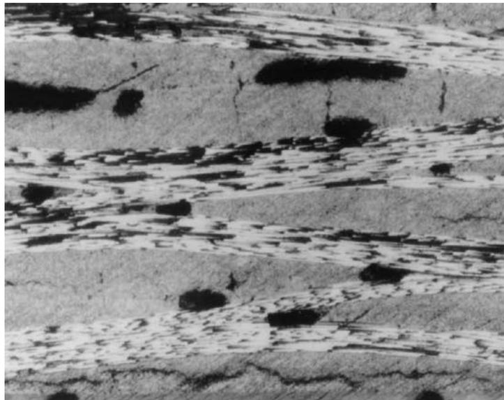
Figure 3 Section of CFRP cured at 400°C.
