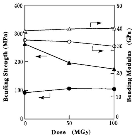
Figure 8 Radiation-resistant property of SiCFRP (MSP). ( $\Delta$ ,  $\blacktriangle$ ): cured at 200°C for 2 hours, ( $\circ$ ,  $\bullet$ ): cured at 400°C for 2 hours.
