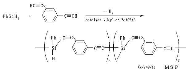
Figure 1 The reaction scheme for the preparation of MSP.
