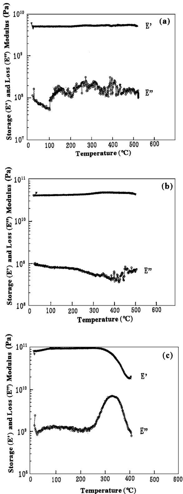
Figure 6 Dynamic viscoelasticities of MSP (a), CFRP (b) and FRP (PMR-15) (c).
