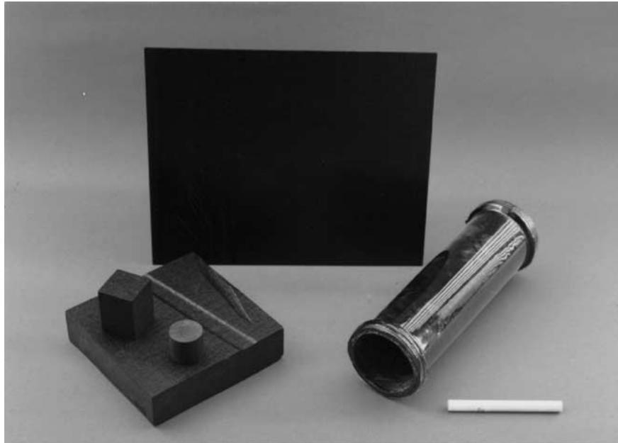
Figure 2 FRPs using MSP as a matrix resin.
